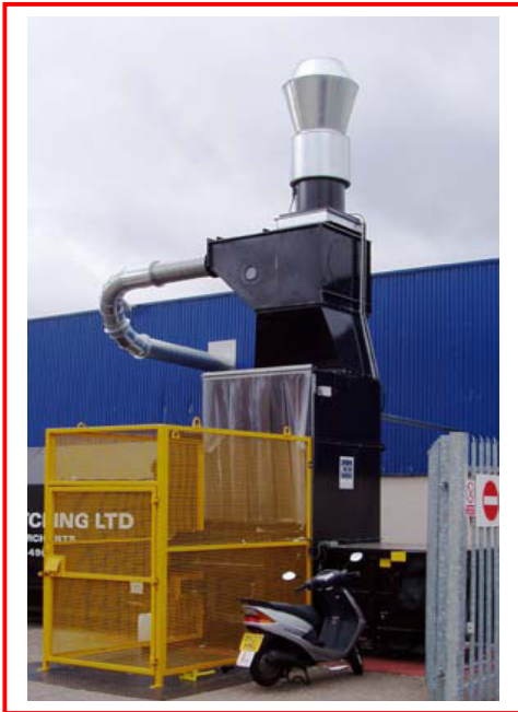
Separator, Compactor and Side Loader
