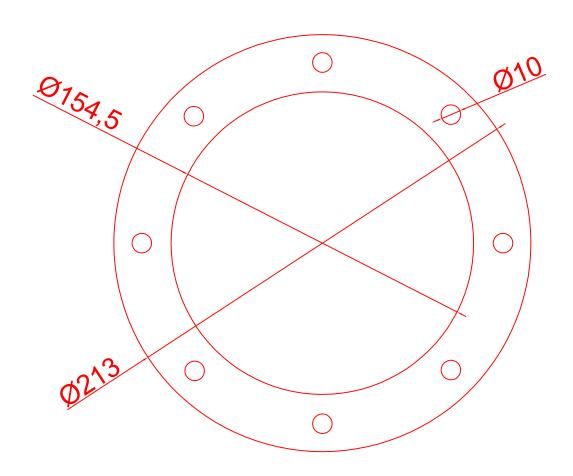
150 Diameter flat bar flange 5mm thick 8 x 10mm holes PCD 189mm Weight 0.68 Kg Electro plated
