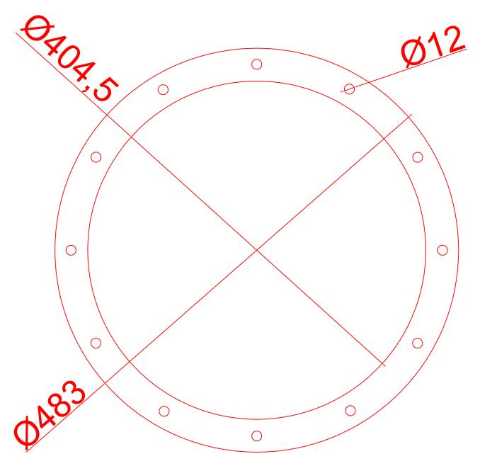
400 Diameter flat bar flange 5mm thick 12 x 12mm holes PCD 454mm Weight 2.18 Kg Electro plated
