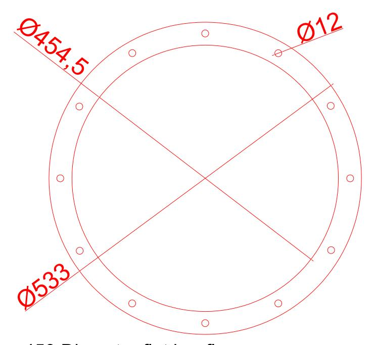
450 Diameter flat bar flange 5mm thick 12 x 12mm holes PCD 505mm Weight 2.43 Kg Electro plated
