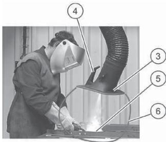
Figure 6-2 Position exhaust hood
