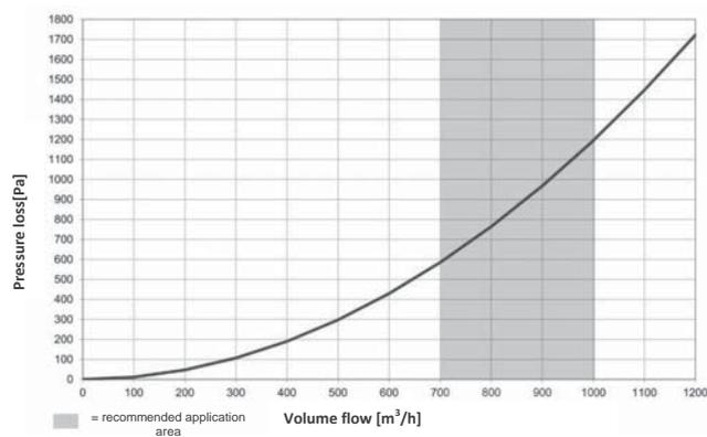
The pressure loss diagram shows approximate values in a normal working position of the extraction arm, which deviate from the diagram values in practice depending on the positioning of the extraction arm.
